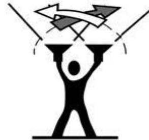
LZ UNSAFE (NIGHT)
