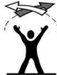
LZ UNSAFE (DAY)
